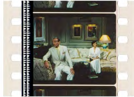
4.17 – Dual unilateral variable area optical soundtrack on 35mm film ( The Band Wagon , Vincente Minnelli, US 1953).
